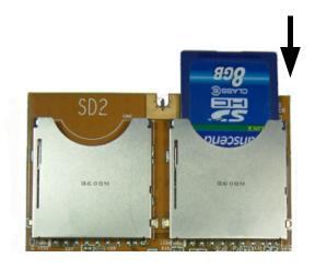
A. Insert SD card into slot
