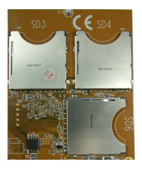
2.2.4 Insert the SD cards into the SD slots in the order indicated (SD1→SD2... SD6)
